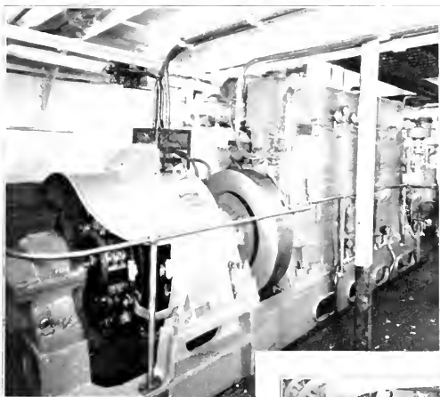
Five views of the machinery on the Columbine. Upper left: The Allan Cunningham winch and control forward of the pilot house on the main deck. Upper right: the Almy water-tube steam boiler with Ray oil burner and the outboard side of the Hill diesel auxiliary generating set. Center left: The Hill-Electro Dynamic auxiliary generating set. Center right: switchboards and control stand on the upper grating of engine room. At right: general view of engine room showing Atlas-General Electric diesel electric main propulsion unit.
